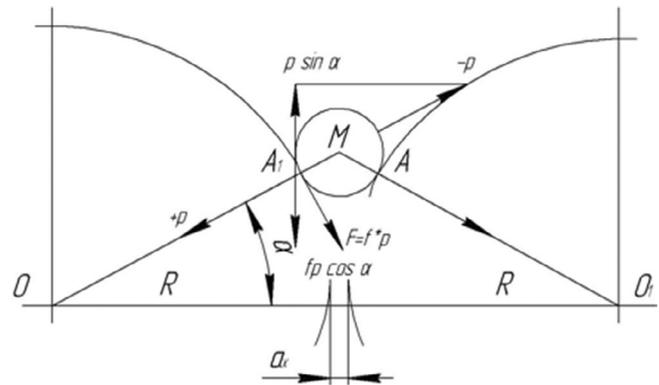
**FIGURE 3** Safflower seed nip scheme with roll mechanism.
