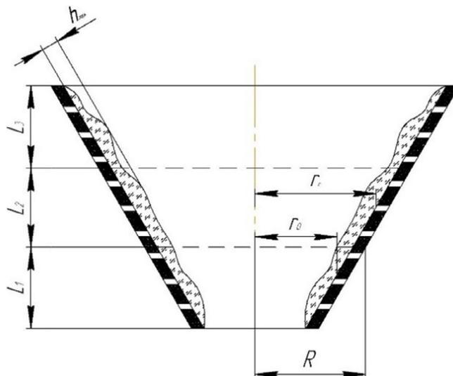
**FIGURE 11** Centrifuge rotor separation areas depending on the separation process.
