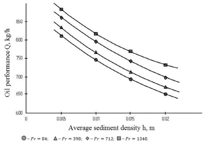
**FIGURE 12** Dependence of oil performance by engineering calculation on average sediment density and various separation factors.
