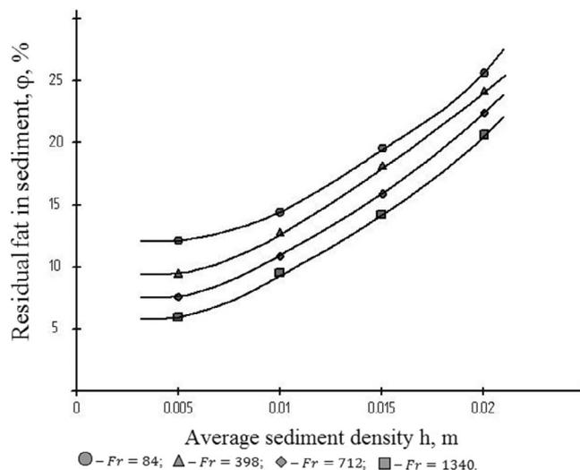
**FIGURE 14** The dependence of residual fatness in the engineering calculation of the mean sediment thickness and various separation factors.
