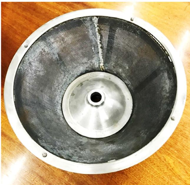
**FIGURE 6** Perforated filter rotor.
