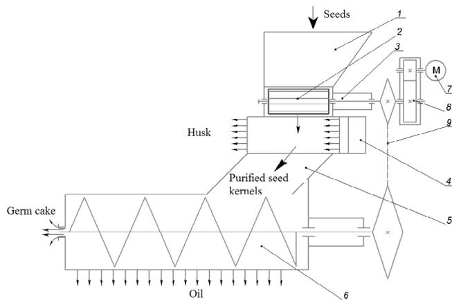
**FIGURE 2** The structural scheme of sheller-compress for oil separation. 1 – bin; 2 – sheller; 3 – roller-type mechanism; 4 – fan separator; 5 – tray; 6 – screw extruder; 7 – electric moto; 8 – reducer; 9 – chain transmission.
