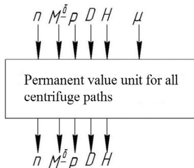
FIGURE 8 Permanent value unit for all centrifuge paths.
