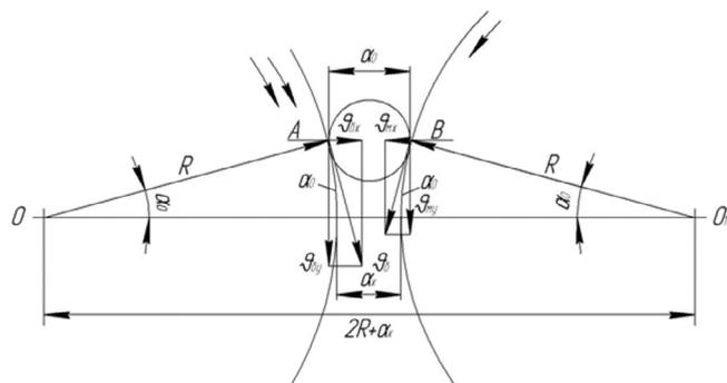
**FIGURE 4** Distribution of the circumferential velocities of the roller mechanism along the axes of coordinates (to determination of the husking duration).  $\alpha_0$  – initial value of the angle of nip  $\alpha$ .
