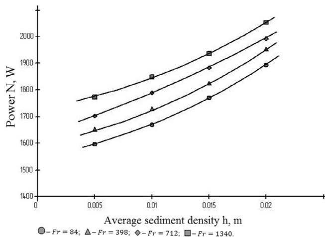
**FIGURE 13** Ratio of engineering power to average sediment thickness and various separation factors.
