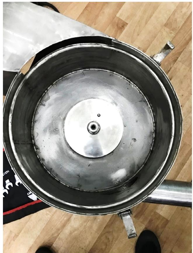
**FIGURE 7** Rotor sedimentation tank.
