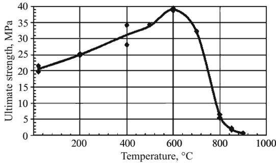
**Fig. 1.** Ultimate strength of a fireclay refractory (ShB-5) in compression versus temperature.
