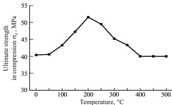
Fig. 4. Ultimate strength  $\sigma_c$  in compression versus temperature.
