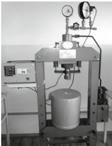
Fig. 3. Setup for measuring the temperature dependence of the ultimate strength in compression.
