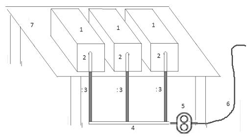
Figure 1 – System for collection of volatile compounds excreted from Colorado potato beetle. Note: 1-chambers; 2-branch pipe; 3-columns filled with activated charcoal; 4-collector; 5-pump; 6-hose; 7 – table
